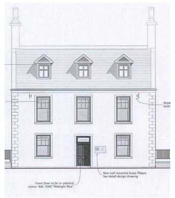
Fig. 6: Proposed brass plaque on the front elevation
